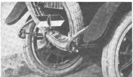
Kruse direction signal on car
